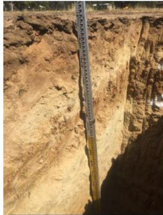
Testhole #2 – with staff showing soil profile depth.
