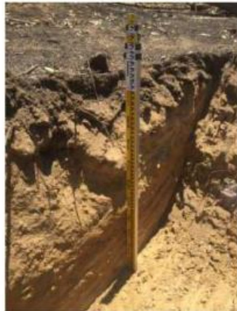
Testhole #5 – with staff showing soil profile depth.
