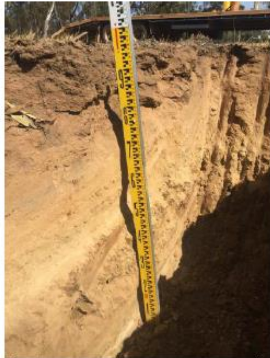
Testhole #1 – with staff showing soil profile depth.
