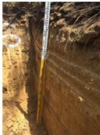
Testhole #6 – with staff showing soil profile depth.
