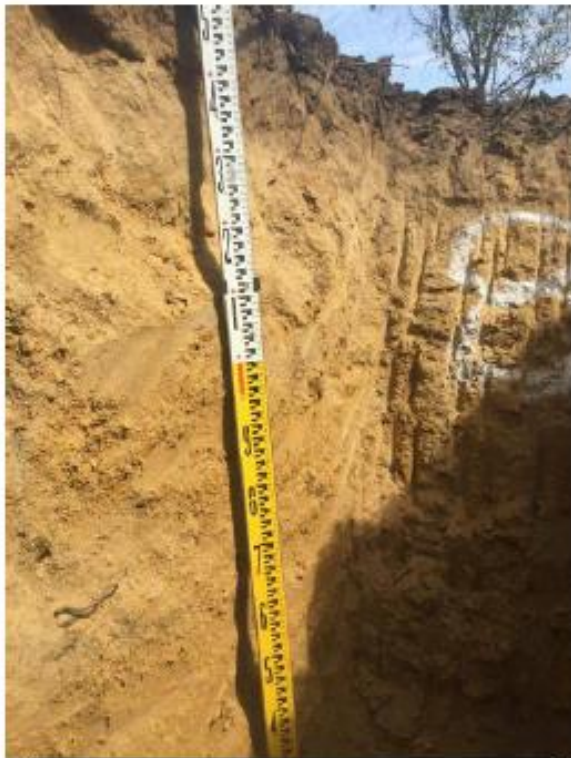
Testhole #8 – with staff showing soil profile depth.
