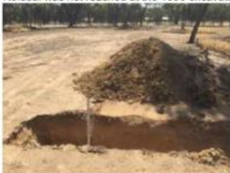
Testhole #2 – with excavated material
