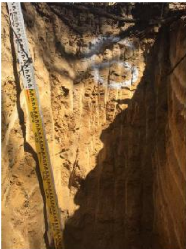
Testhole #6 – showing sample excavation locations.
