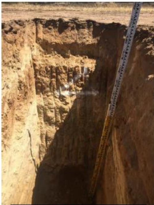
Testhole #2 – showing sample excavation locations.
