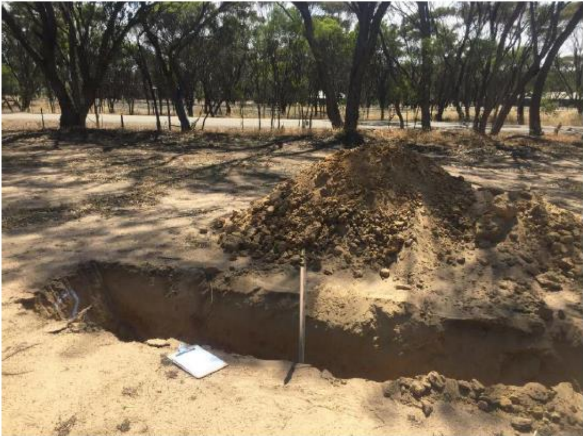
Testhole #3 – with excavated material
