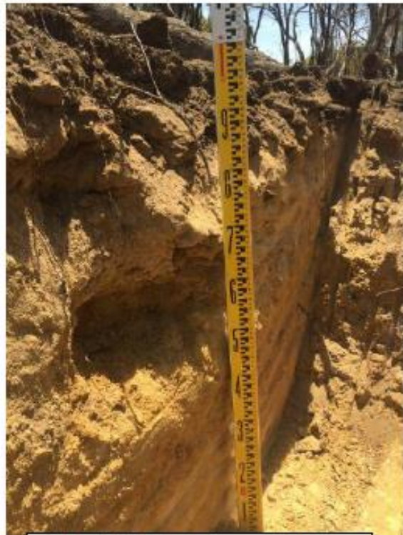
Testhole #5 – showing sample excavation locations.
