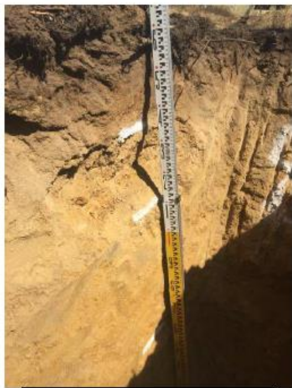
Testhole #8 – showing sample excavation locations.
