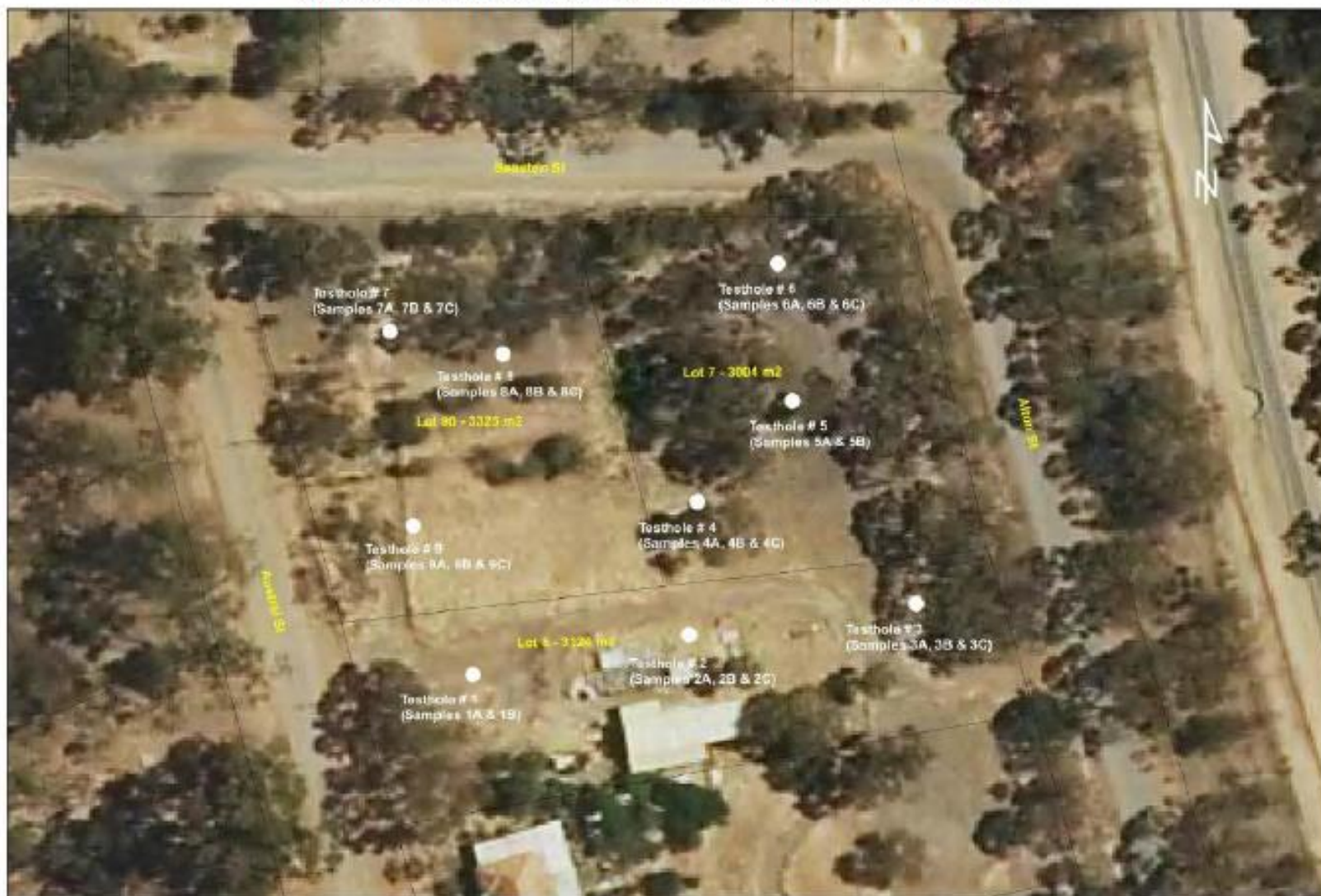
Site Plan for Site Classification Soil Sampling on 3 Lots in Cuballing
