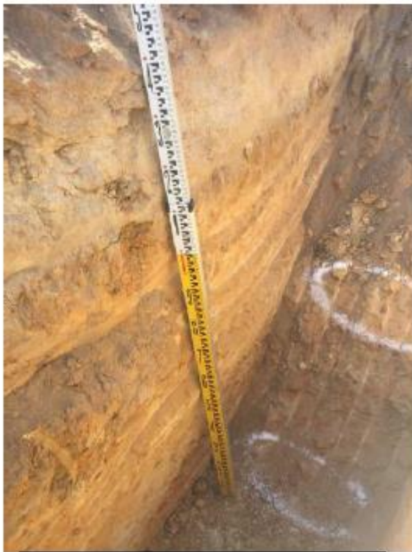
Testhole #9 – with staff showing soil profile depth.
