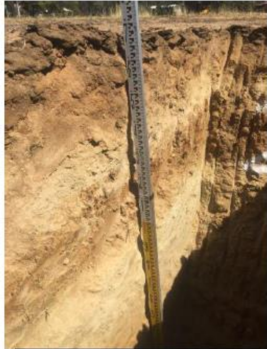
Testhole #2 – with staff showing soil profile depth.
