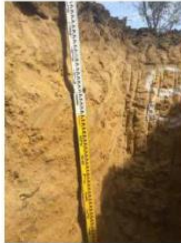
Testhole #8 – with staff showing soil profile depth.
