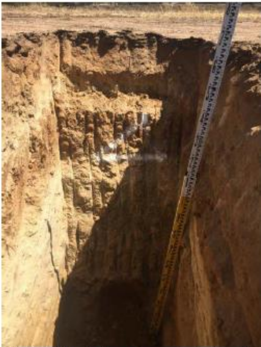
Testhole #2 – showing sample excavation locations.
