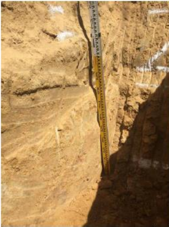
Testhole #7 – with staff showing soil profile depth.
