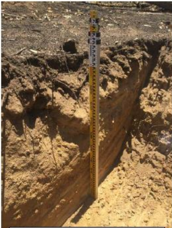
Testhole #5 – with staff showing soil profile depth.
