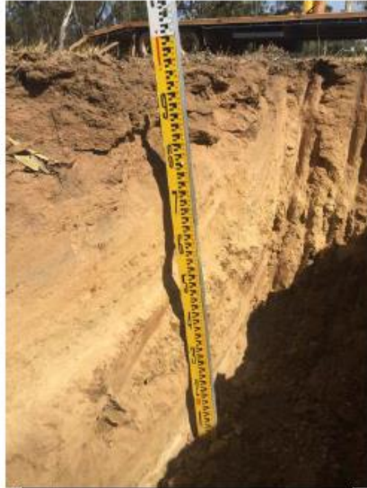
Testhole #1 – with staff showing soil profile depth.
