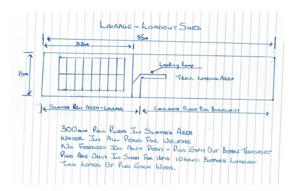
The shed is built of 200mm H beam posts and trusses. They are hot dipped galvanised as are all of the other sheds we have built recently. The roof will be zincalume trim-deck. We normally put insulation panel on our sheds to keep the heat out. We do not need to do it for this one as the pigs will only go into the shed the night before they are trucked. There are also no walls on this shed.
